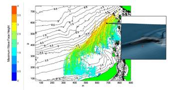
OPTISURF calculates surf-ability using a detailed wave-by-wave approach. It produces hourly statistics of the distribution of ride length, wave pealing speed, and wave face height. © DHI
