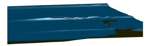
Coupling the MIKE 21 BW Boussinesq wave model to a fully non-linear CFD model allows for detailed assessment of wave breaking characteristics along famous surf breaks around the world. © DHI
