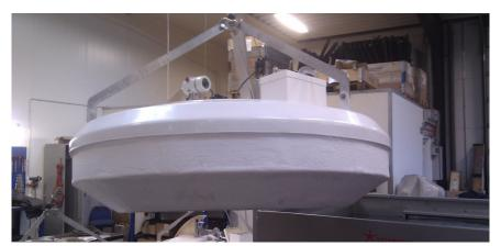
A specially designed off-gas unit is an essential part of the DHI monitoring unit for waste water treatment plants. ©DHI /Stjernholm
