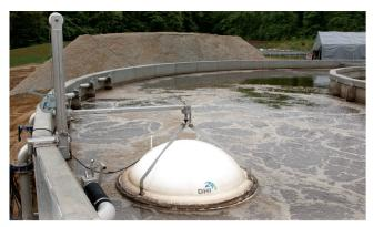
During testing, the off-gas unit will be placed at the surface of the tank where the biological treatment process takes place. © DHI
