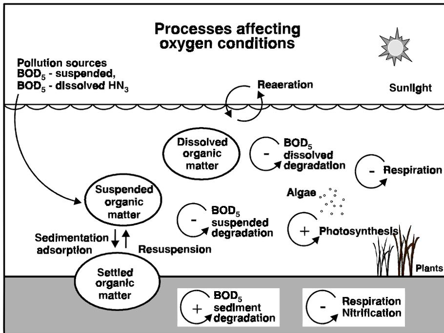
Figure 5.1 Principle sketch of BOD/DO model
