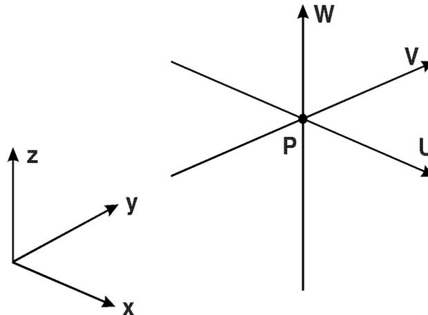
Figure 2.2 Definition of the prognostic variables used in the hydrodynamic part of MIKE 3
