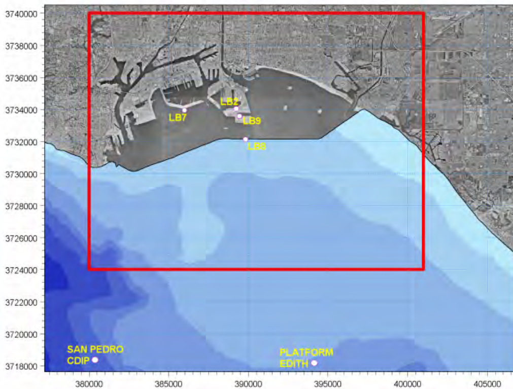
Fig. 8. Location of wave gages. The rectangle indicates the boundaries of the MIKE 21 BW model. Co-ordinates are UTM zone 11
