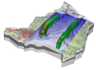
3D well capture zone (red/green isosurfaces) and mean life time expectancy (blue isosurfaces).
