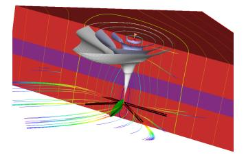
3D capture zone of a Ranney collector well (combination of vertical and horizontal well screens).
