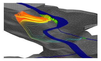
Visualisation of water sources (bullets), flow traces and travel times for a pumping well.
