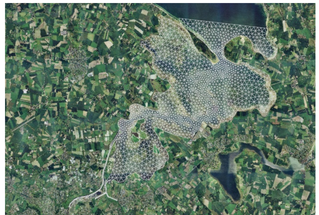
2D visualization of a computational mesh (Odense Estuary)
